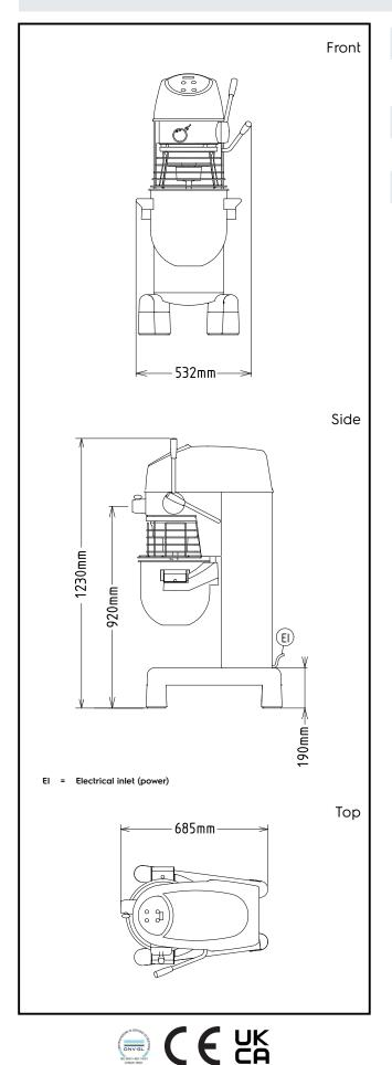
**Electric** Supply voltage: 200-240/380-415 V/3 ph/50 600231 (XBM20AXB3) Capacity: Performance (up to): 6 kg/Cycle Capacity: 20 litres
